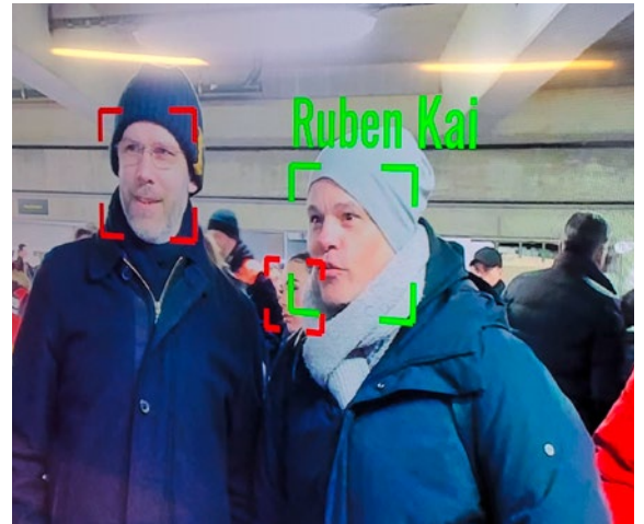
Demonstration of facial recognition. Green means the face is recognised and the person is accredited. Red means the face is recognised and the person is not accredited.
